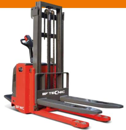
The brake override, feature on MIMA stackers allows travel (creep speed) with the handle in a near vertrical position while staying within the geometry of the truck. This provides exeptional manuverability in extremly restricted areas.
